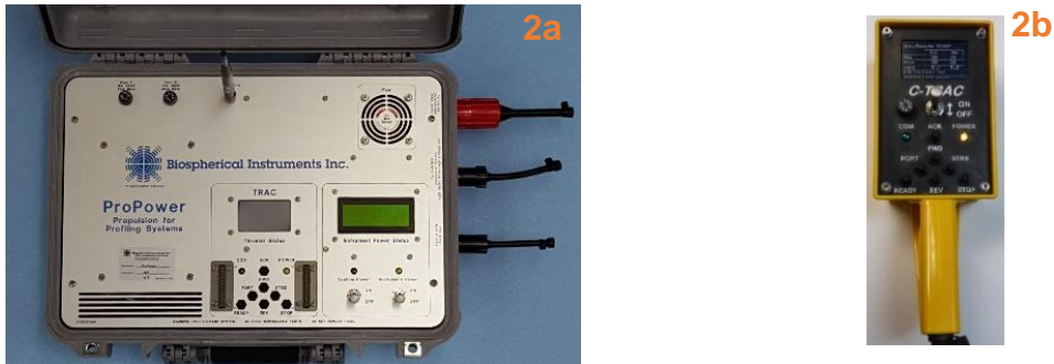
Fig. 2. C-PrOPS power and thruster controls; (a) ProPower box with TRAC, and (b) C-TRAC wireless remote-control unit.
