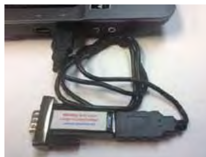
Figure 1. The BSI USB-to-serial adapter, with the DB9 serial connector, is shown with BSI's customized labels on either side of it. Top: The adapter is plugged directly into the laptop's USB port; the label says to connect it only to BSI Instruments (referring to the side of the adapter with the DB9). Bottom: The reverse side of the same adapter is shown plugged into an extension cable; the warning label says that the serial output voltage has been modified.
