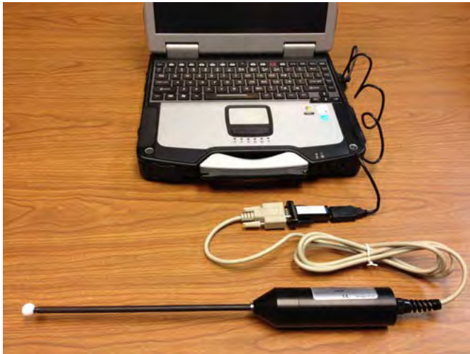
Figure 2. The USB-to-serial adapter (middle of photo) is shown properly configured with the laptop and one of BSI's Q-series instruments, the QSL-2101.
