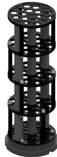
Fig. 18. A drawing of the four layers of Gershun tubes, and baffle placement for a 2.5^\circ FVA.
