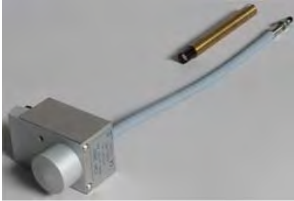
Fig. 37. The Zeiss/Tec5 MMS spectrograph with the fiber optics shown alongside a microradiometer for scaling purposes. A fully assembled microradiometer, with metal sleeve and front-end optics, has a dimension of 0.435 \times 3.79 \text{ in}^2 .
