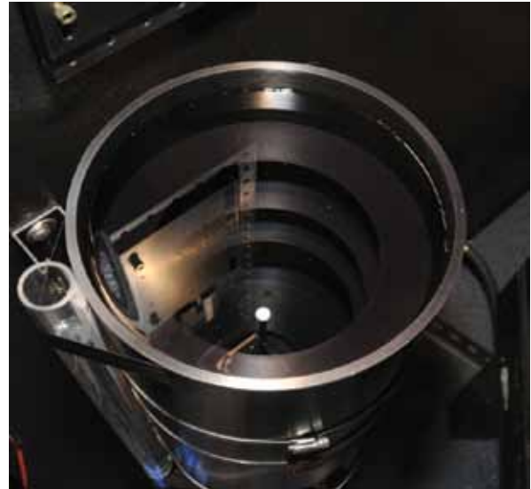
Figure 2. AMOUR scalar irradiance collector immersed in water inside a tank designed for accurate determinations of immersion coefficients. The small cylinder at the left is a sight glass to determine the water level. Internal baffles suppress stray light, and an aperture (not shown) is normally installed at the top of the container.
