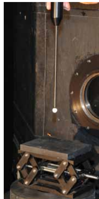
Figure 4. AMOUR probe taking the baseline reading at the reference position in air.
