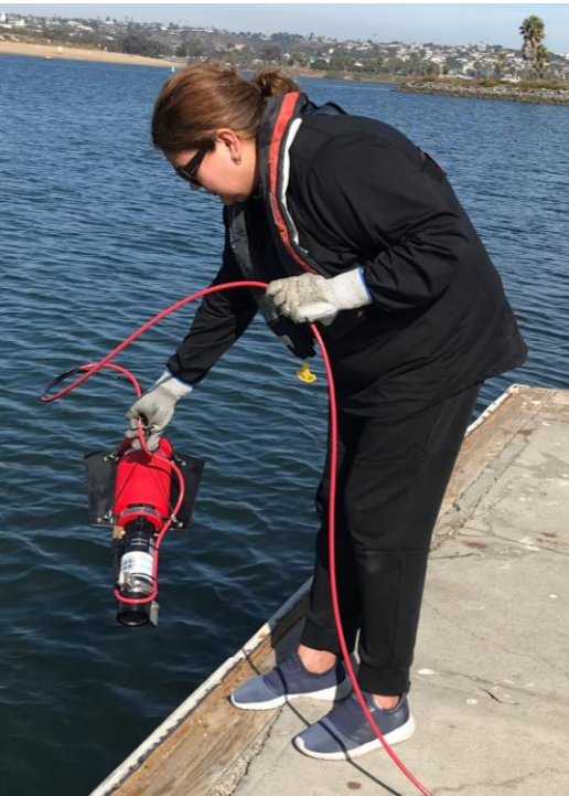
Figure 1. The XRL is small, lightweight, and easily hand deployed using a free-fall float collar (shown in red). The radiance end of the instrument can be seen at the bottom of the cylindrical housing.
