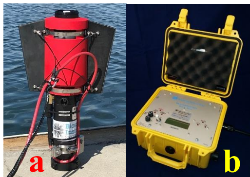
Figure 3. (a) An XRL with E_d and L_u geometries sharing a single 46 cm long housing. The XRL or the XRE are typically deployed using a unique hydrobaric free-fall collar, known as X-SLOWS (shown in red). X-SLOWS can be optimized for slow descent rates for work in very shallow coastal waters, or faster descent rates for observations in the open ocean. (b) An XTRA-class microradiometer deck box supplies power and RS-485 telemetry to the XRR system, and USB communications to the data acquisition computer.
