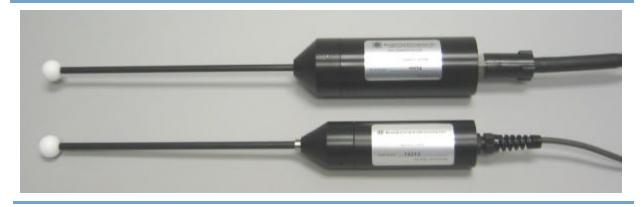
The QSL-2100 quantum scalar sensor features a 1.9 cm diameter Teflon® spherical optical collector and is designed to provide accurate measurement of photosynthetically active irradiance (PAR) in aquatic or dry environments. The small size of the scalar collector and convenient hand wand ensure that Biospherical Instruments' QSL sensors provide accurate light measurements from virtually all directions.
