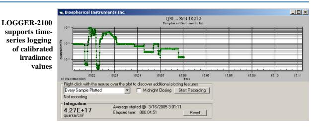
**Software:** LOGGER-2100 software is included with each sensor and is compatible with Windows 7, VISTA and XP. Data are in PC compatible digital format. The user may configure output for display in Quanta or Microeinsteins.
