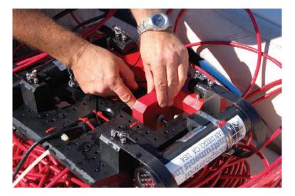
The C-OPS near-surface buoyancy is easily adjustable using a combination of air filled and rigid foam floats. As the system descends, the increasing water pressure compresses air-filled bladders, which reduces buoyancy and increases the descent rate from <3 cm s<sup>-1</sup> at the surface, to over 30 cm s<sup>-1</sup> below 10 m.
