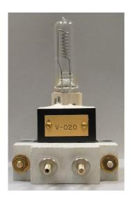
Calibrations performed at Biospherical Instruments are traceable to the scale of spectral irradiance maintained by the National Institute of Standards and Technology (NIST). NIST distributes this scale in the form of 1000 W tungsten-halogen lamps of type FEL. An article describing how this scale is maintained at BSI is <u>here</u>.
