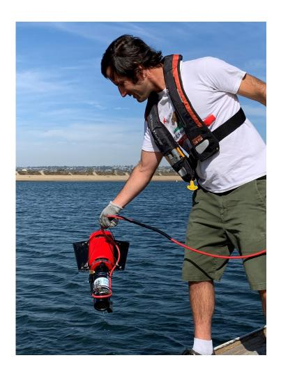
Biospherical Instruments Inc (BSI) has released the newest member of the Expandable Technology for Radiometric Applications (XTRA) class of high performance field instruments called the <a href="XTRA Reflectance Radiometers">XTRA Reflectance Radiometers</a> ( XRR ) . The XRR is an economically priced multiwavelength radiometer for determining apparent
