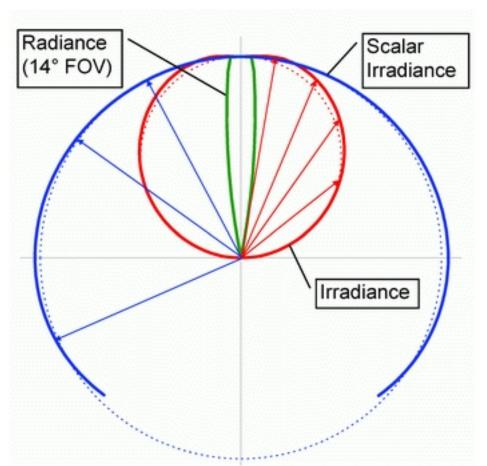
Biospherical radiometers are available with a variety of light collection geometries. With the AMOUR device, the user can select from the following measurement geometries. Calibration data for every type is available.
