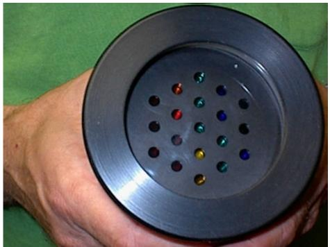
**Radiance** sensors are easy to identify because they do not typically have a diffuser (**Figure 1**). In our systems, filtered photodetectors are positioned at the bottom of individual Gershun-style tubes, which restricts the field-of-view to the desired solid angle. Radiance is typically a bbreviated with the symbol *L*.
